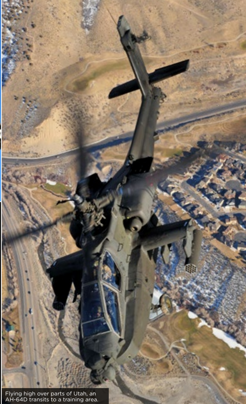
The wings of the Apache can carry multiple types of weapons, including rockets and Hellfire missiles.
