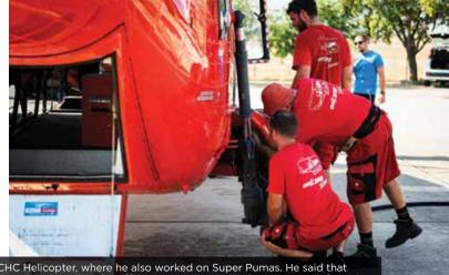
Certifying engineer Jean-Louis Leveau came to Heli Austria from CHC Helicopter, where he also worked on Super Pumas. He said that maintenance on the aircraft for heavy-lift applications is somewhat more intensive than for offshore operations: "We have some reinforced inspections because it's a lifting aircraft. Especially the tail boom has to be checked a bit more, and the sling also has to be checked very often."
