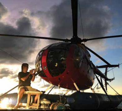
Bob repairs a cracked chin bubble on the MD 500 at the end of a long day's work.
