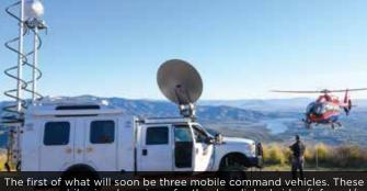
serve as mobile signal receivers for the downlinked video/infrared/ ultraviolet signals from the FLIR Corona 350 II. They can also be sourced at no cost for appropriate public safety missions
