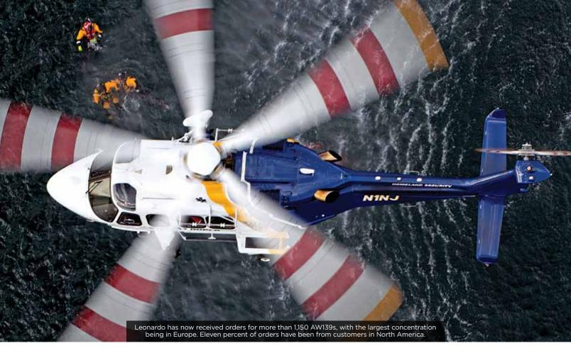
Leonardo then introduced an 882-lb. (400-kg) increased gross weight option in 2008, which lifted the MTOW from 14,110 lb. to 14,991 lb. (6,800 kg), and at Heli-Expo 2015, announced a seven-tonne (15,431-lb./7,000-kg) increased gross weight kit that could be introduced on new production and in-service aircraft.
