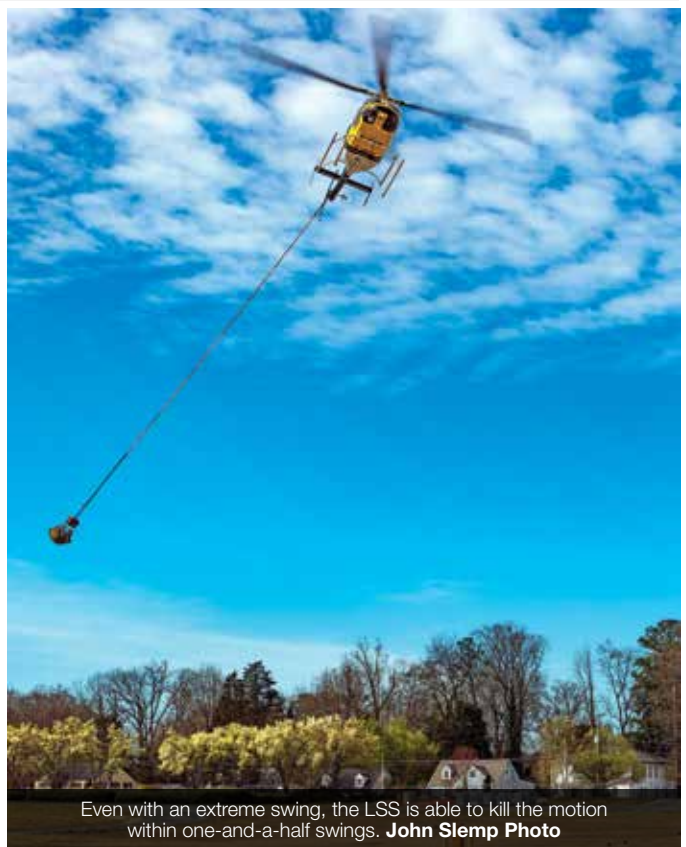
Vita Inclinata used a Bell 407HP operated by Helicopter Express for the first public flight demonstration of the LSS. John Slemp Photo
