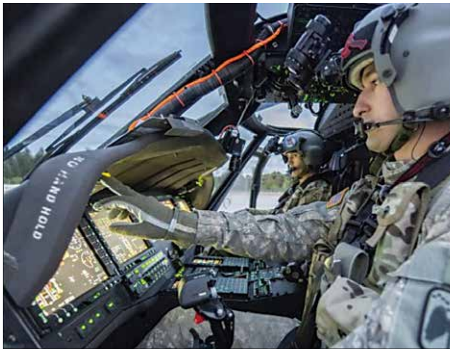
Aircrews conduct final pre-mission checks for a nighttime air assault mission during operational tests of Army modernization efforts with a new digital cockpit in the UH-60V Black Hawk. Tad Browning Photo
