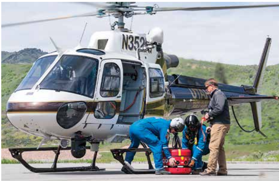
Since receiving the Recco SAR Helicopter Detector just under a year ago, Utah DPS has deployed the system on three avalanche incidents, and was successful in locating the victim each time.
