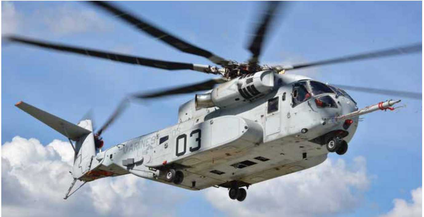
Collins Aerospace is the supplier for the complex drive system on the CH-53K, which has three engines and a folding tail boom. Mike Reyno Photo
