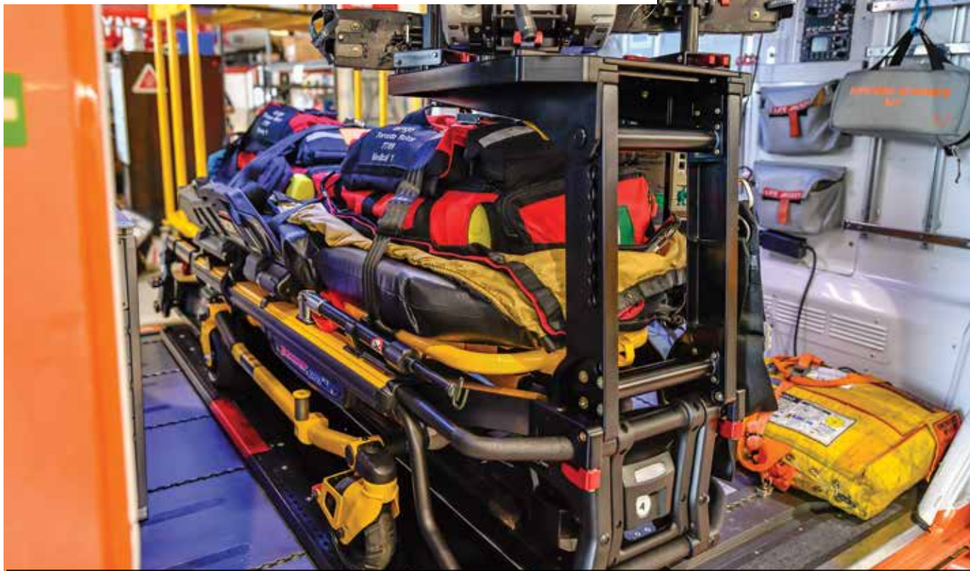
Ornge has completed the installation of the HeliMods PAL stretcher system across its fleet of 11 Leonardo AW139s. Rob Reyno Photo
