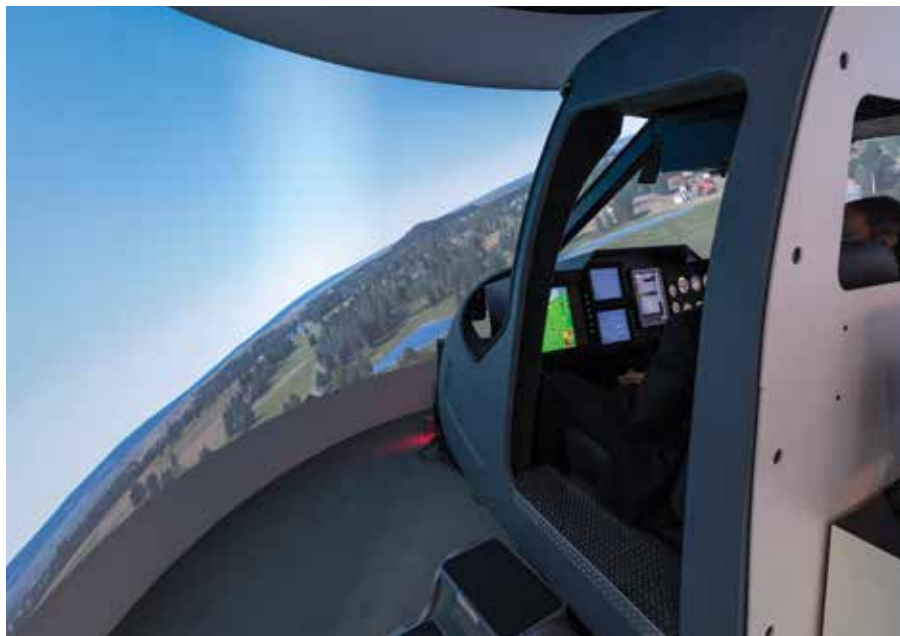
The simulator module on display at DSEI was a generic Airbus EC135 cockpit, with imagery directly projected onto a half dome. Garry Ridsdale Photo
