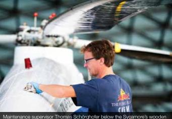
rotor blades, which are visually inspected before and after each flight.
