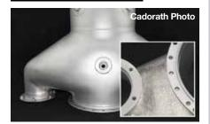
Cadorath, in partnership with Rolls-Royce, has announced the design and approval to provide repairs and overhauls to the M250 Series IV outer combustion case (OCC). Overhauls will include repairs to the fuel boss and replacement of the existing wire mesh patches with new reinforced dual wire mesh patches.
