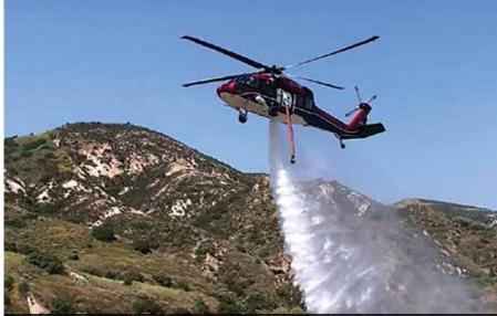
The internal fire attack system allows the Black Hawk to carry 900 US gallons of water or foam. Simplex Photo
