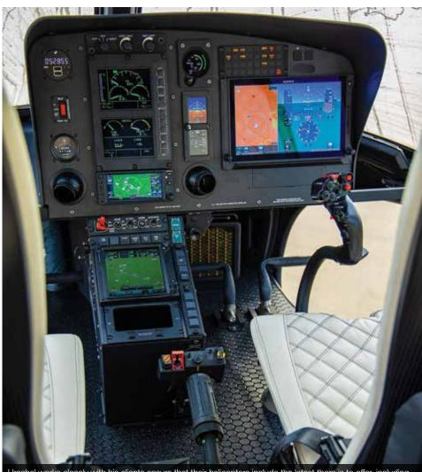
Urschel works closely with his clients ensure that their helicopters include the latest there is to offer, including avionics. In this case, Hangar One Avionics customized an H125 avionics panel with a 10.6-inch Garmin G500H TXi touchscreen flight display, Garmin GTN 750 and TN650 that combines GPS, communication and navigation functions.
