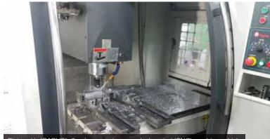
Pictured is ICARUS's 3-axis computer numerical control (CNC) machine, which assists with production and manufacturing of airframe parts and components.
