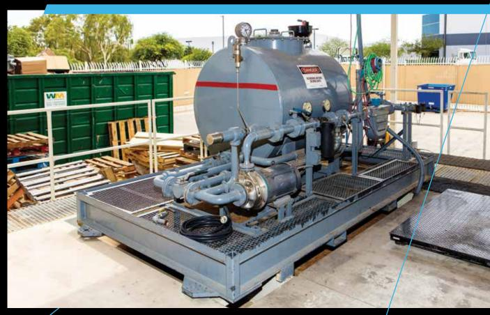
After each tank is assembled, it is connected to this unit for acceptance testing, which checks for leaks and ensures correct gauging and pump operation. Each acceptance test usually lasts between one and one-and-a-half hours, and uses a special solvent, rather than jet fuel, for safety and environmental reasons.
