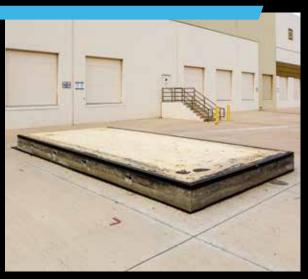
The concrete pad where Robertson conducts its drop tests. The FAA requires that tanks be dropped from a height of 50 feet while 80 percent full of water (approximating the mass of the tank full of jet fuel, which has a lighter density than water). The U.S. military generally stipulates that tanks be dropped full of water from at least 65 feet, but does not require that they be dropped in a representative aircraft structure.
