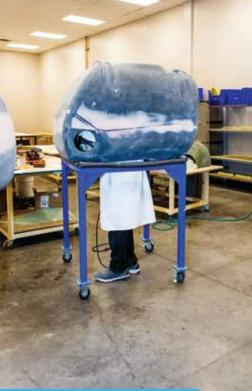
Robertson makes the composite container for the H125/AS350 CRFT in-house using preimpregnated carbon fiber and fiberglass.
