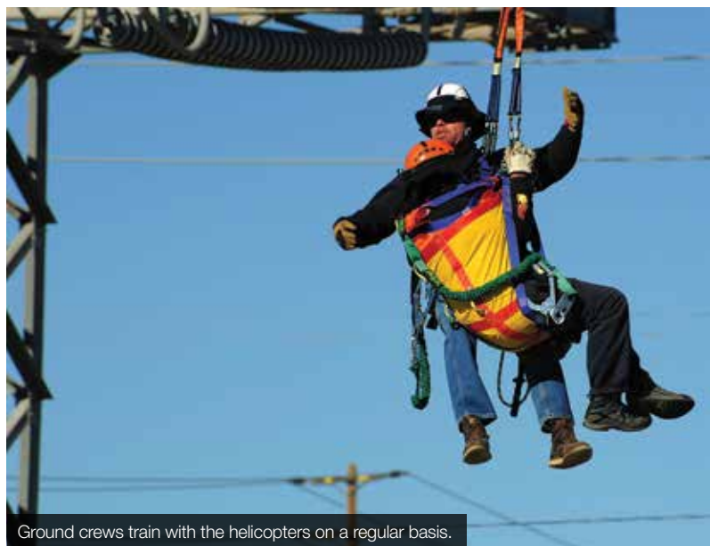
Dual hooks from Boost Systems are used for the human external cargo (HEC) operations.
