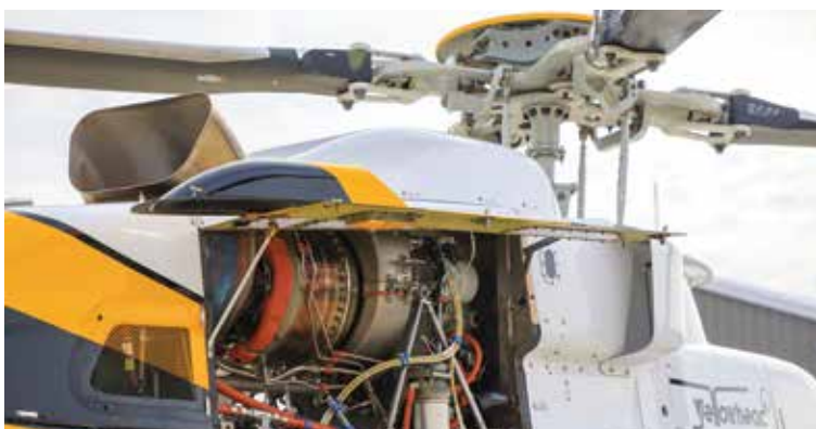
A look under the cowling of an Eagle 407HP, which replaces the Bell 407's Rolls-Royce 250-C47B engine with a Honeywell HTS900-2. Heath Moffatt Photo
