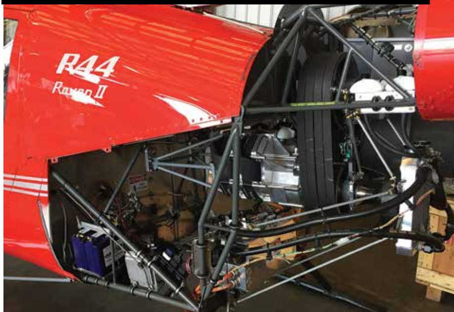
The aircraft's twin electric motors are stacked together and provide redundancy in the event of a motor failure. "We're basically flying a twin, if you want to look at it that way," said Ric Webb. Tier 1 Photo
