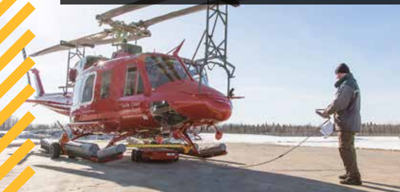
A V614 Universal Tow Cart moves a Canadian Coast Guard Bell 412EP1 helicopter. The V614 was initially designed to be operated through a remote control attached by a wire, but the company released a wireless version in 2017.
