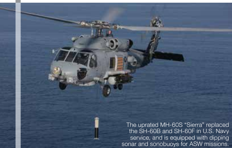
The MH-60S has a blend of UH-60M and MH-60R attributes. It has two doors on each side, a tail wheel, and an MH-60R rotor head and avionics to achieve as much cockpit commonality as possible. Skip Robinson Photo
