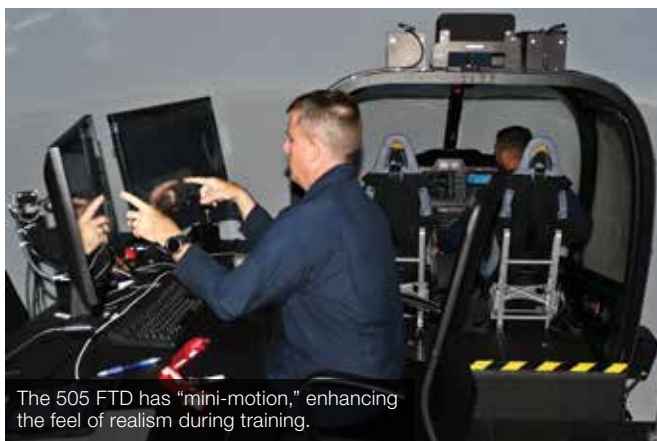
A student takes the controls in the Bell 505 flight training device. The device was created by Textron sister company TRU Simulation & Training, and went into operation in July 2018.
