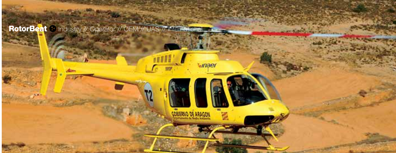
The Solar Advantage windshields and windows are said to improve the blocking of ultraviolet rays and reduce infrared and solar radiation. Bell Photo
