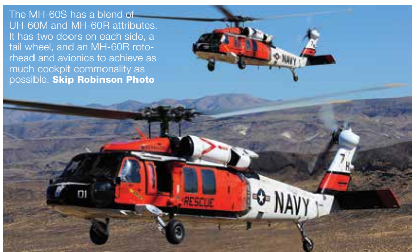
The updated MH-60S “Sierra” replaced the SH-60B and SH-60F in U.S. Navy service, and is equipped with dipping sonar and sonobuoys for ASW missions.
