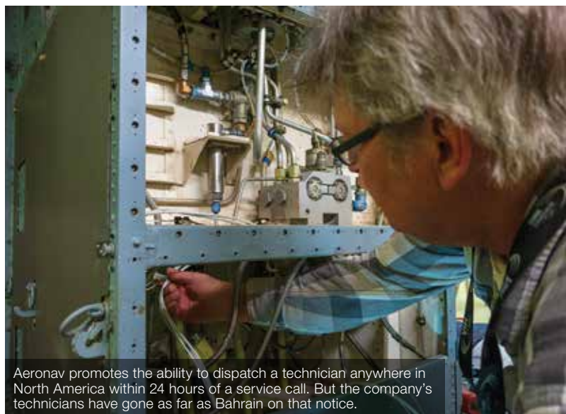
Aeronav's Carinha spools a 22 AWG wire into the company's laser wire marker. The wire will be used for a Sikorsky S-61N helicopter's ELT system.
