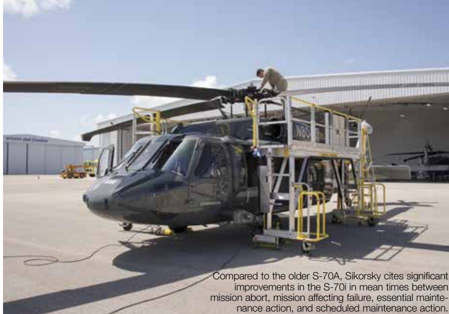
The S-70i has automatic diagnostics for main rotor blade tracking and balancing. The new blade design has also eliminated BIM pressure indicators.
