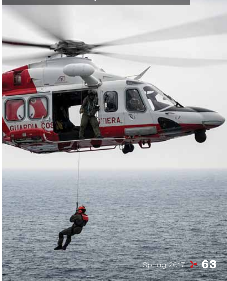
Guardia Costiera's AW139s are equipped with Breeze-Eastern electric rescue hoists. The helicopters' elongated noses contain weather radar.
