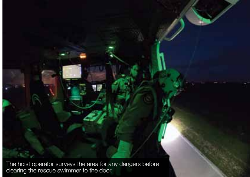
The Guardia Costiera's AW139s are fully equipped for night vision goggle operations.
