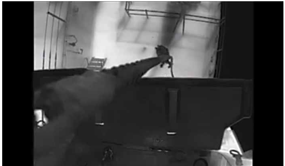
A vertically mounted EVS can provide pilots engaged in hoisting operations with an infrared image of the area below the helicopter, even at night and in bad weather. Lexavia Images
