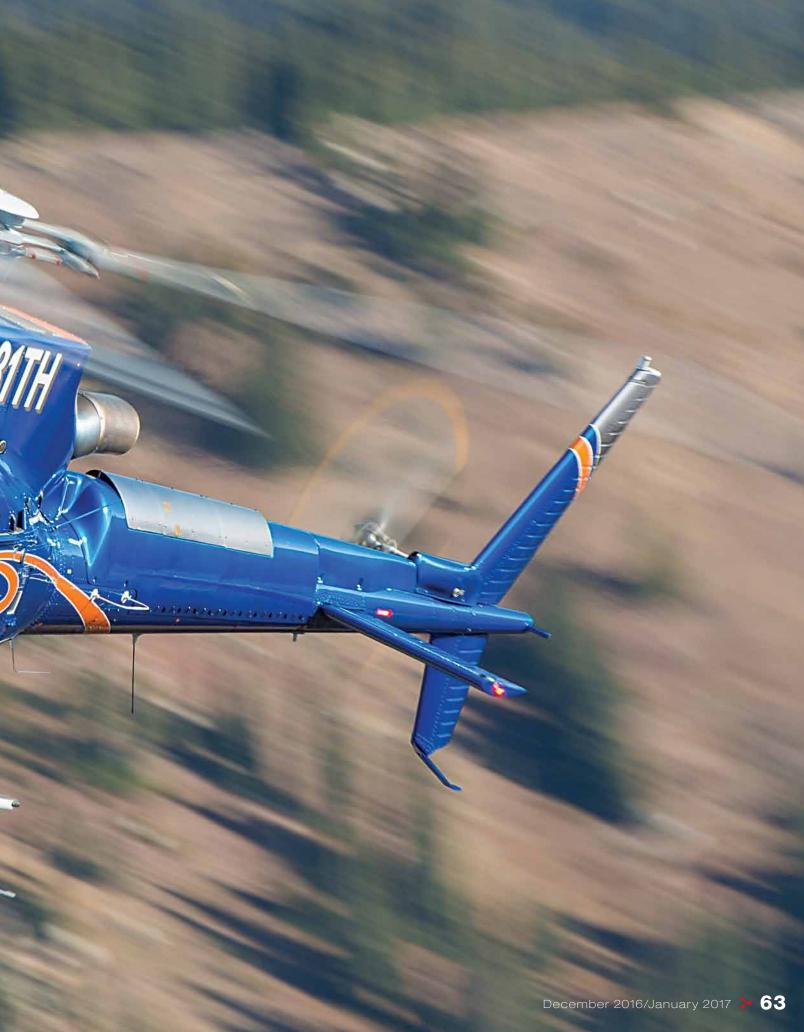
notice any change to the available left pedal authority, even at 80 knots indicated airspeed, where almost all of that pedal authority is used in overcoming the effect of the upper vertical fin.
