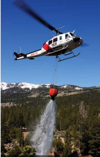
Since this photo was taken, the NDF has upgraded its 240-gallon Bambi Buckets to the more capable PowerFill version that allows the helicopter to use water from many more sources.
