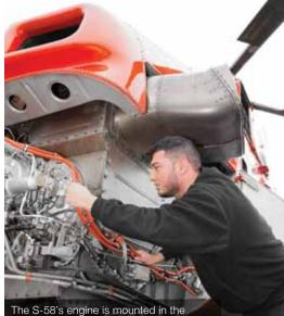
The S-58's engine is mounted in the aircraft's nose. Here, aircraft maintenance engineer Rahmatullah Rahimi takes a look behind the cowlings.
